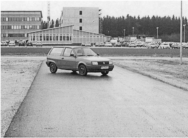
Fig. 9. Car approaching the sensor from forward left-hand side (distance 17 m, speed 8.1 m/s).
