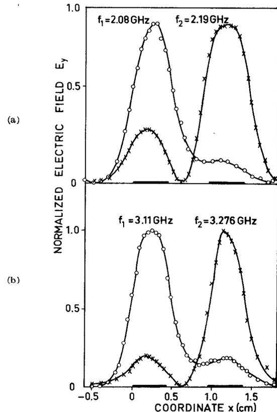
Fig. 2. Field component  $E_y$  of four resonances of the straight double-line resonator with lines of different lengths as a function of the coordinate  $x$ . Resonator dimensions as in Fig. 1,  $\Delta l = 0.4$  cm.
