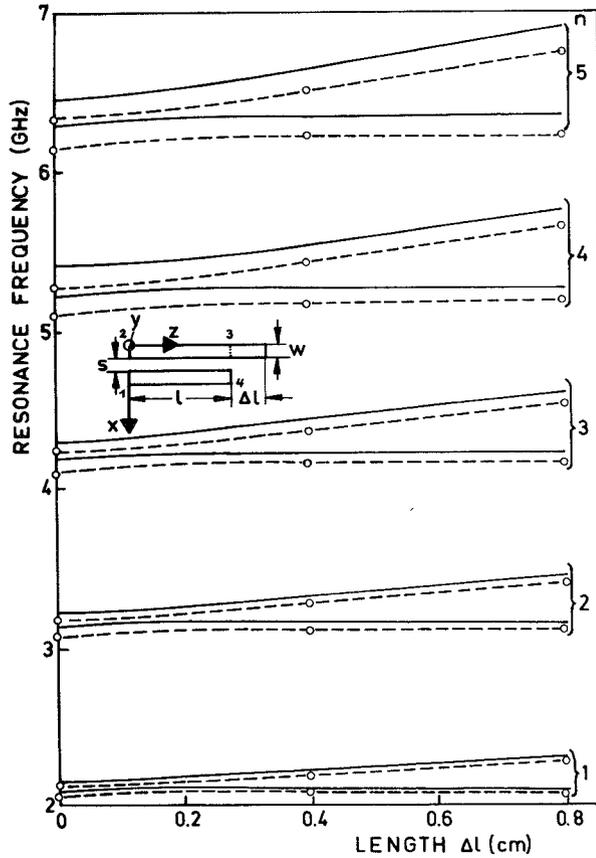
Fig. 1. Resonance frequencies and structure of the straight double-line resonator of constant length  $l + \Delta l$ . Resonance frequencies in dependence on the difference  $\Delta l$  of the line lengths. Substrate material Polyguide ( $\epsilon_r = 2.32$ ,  $h = 0.156$  cm). Resonator length  $l + \Delta l = 10.01$  cm,  $w = 0.44$  cm,  $s = 0.5$  cm.  $\circ$  Experimental results.
