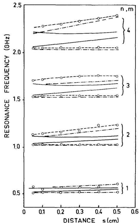
Fig. 4. Resonance frequencies of the double-ring resonator as a function of the distance  $s$  between the rings. — calculated by (4), - - - calculated by (5), —○— experimental results. Resonator dimensions:  $r_4 = 6.84$  cm = const,  $w = 0.44$  cm,  $h = 0.156$  cm. Substrate material Polyguide ( $r_4$  is the outer radius of the outer ring).
