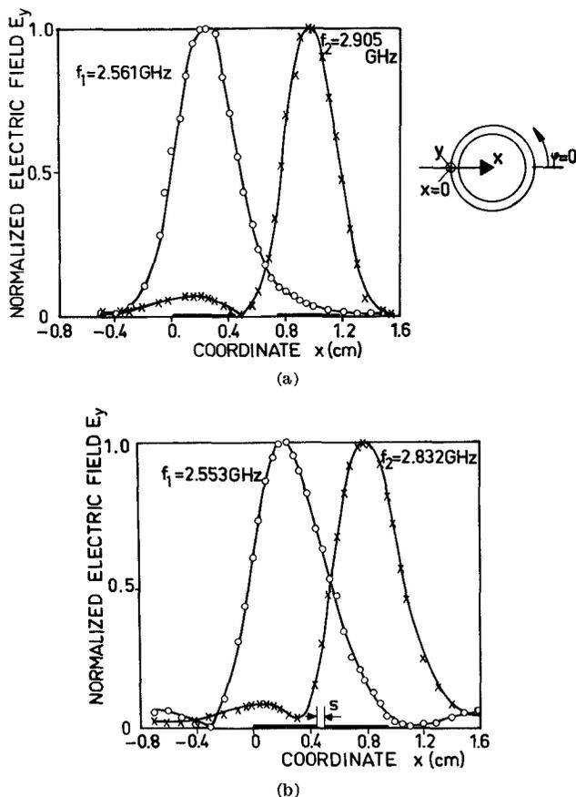
Fig. 3. Field component  $E_y$  of four resonances of the double-ring resonator. (a) Resonator dimensions:  $r_4 = 6.84$  cm,  $w = 0.44$  cm,  $s = 0.30$  cm,  $h = 0.156$  cm. Substrate material Polyguide ( $r_4$  is the outer radius of the outer ring). (b) Resonator dimensions:  $r_4 = 6.84$  cm,  $w = 0.44$  cm,  $s = 0.05$  cm,  $h = 0.156$  cm. Substrate material Polyguide.
