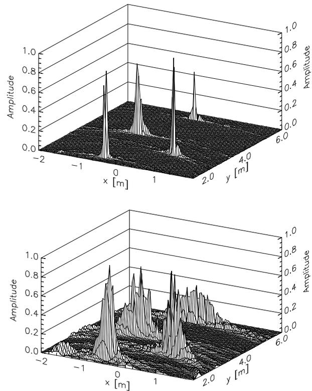
**Fig. 3:** Images of 4 cylinder arrangement according to Fig. 2 with bandwidths of 11 GHz (top) and 1 GHz (bottom).
