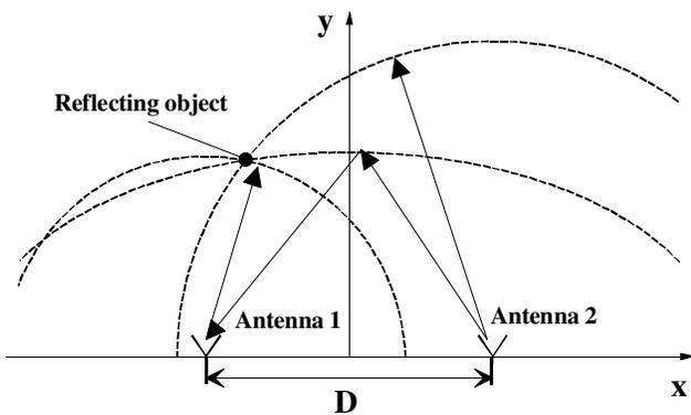
**Fig. 1:** Basic principle of the imaging sensor.
