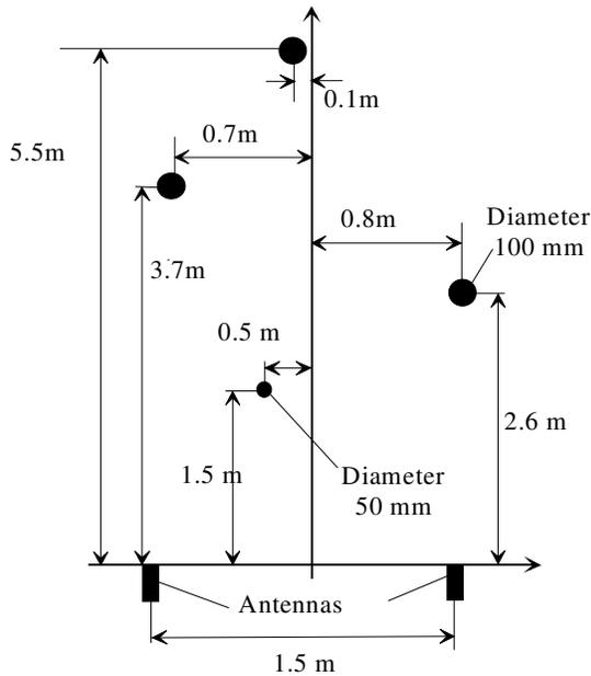
**Fig. 2:** Geometrical arrangement of 4 metal cylinders.
