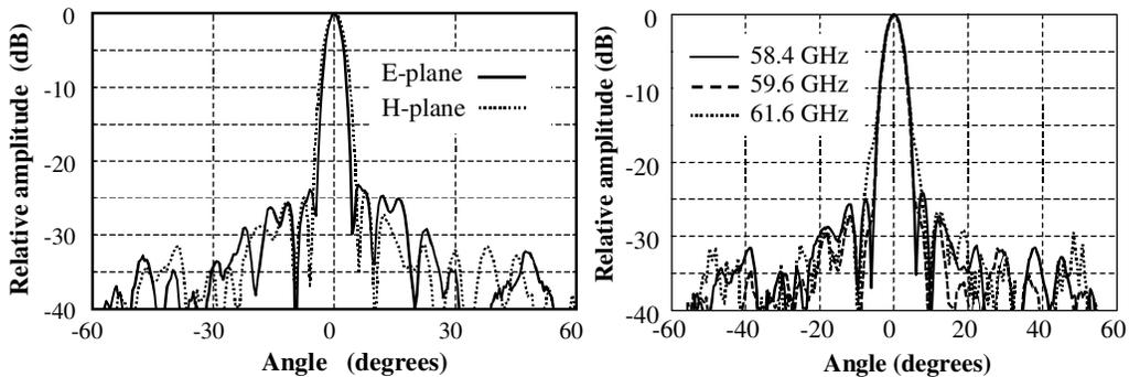
**Fig. 5:** Radiation diagrams of the V-band folded reflector antenna. (Left side: E- and H-plane at 58.4 GHz. Right side: H-plane at 58.4, 59.6, and 61.6 GHz. Reflectarray and grid: Duroid material of 0.254 mm and 1.58 mm thickness, respectively).
