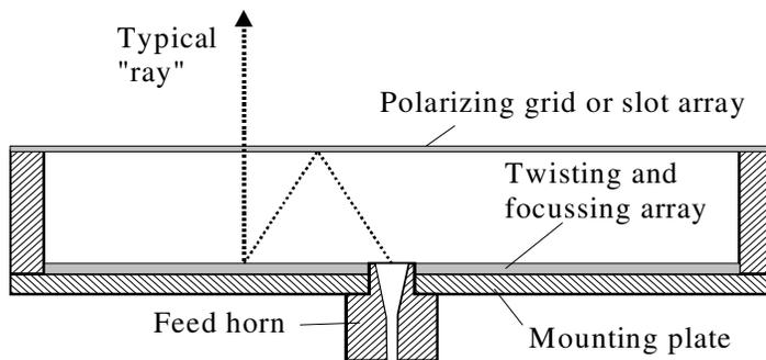
**Fig. 2:** Basic principle of the folded reflector antenna.
