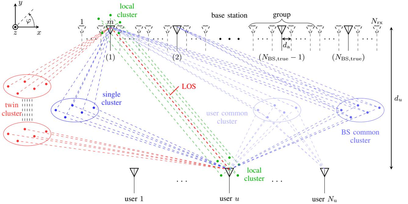
Fig. 2. Overview of the extended COST 2100 channel model for multi-user massive MIMO transmission. Depicted clusters are exemplary for user  $u$  and base station antenna  $m$ . True antennas are drawn in solid and interpolated antennas in dashed.
