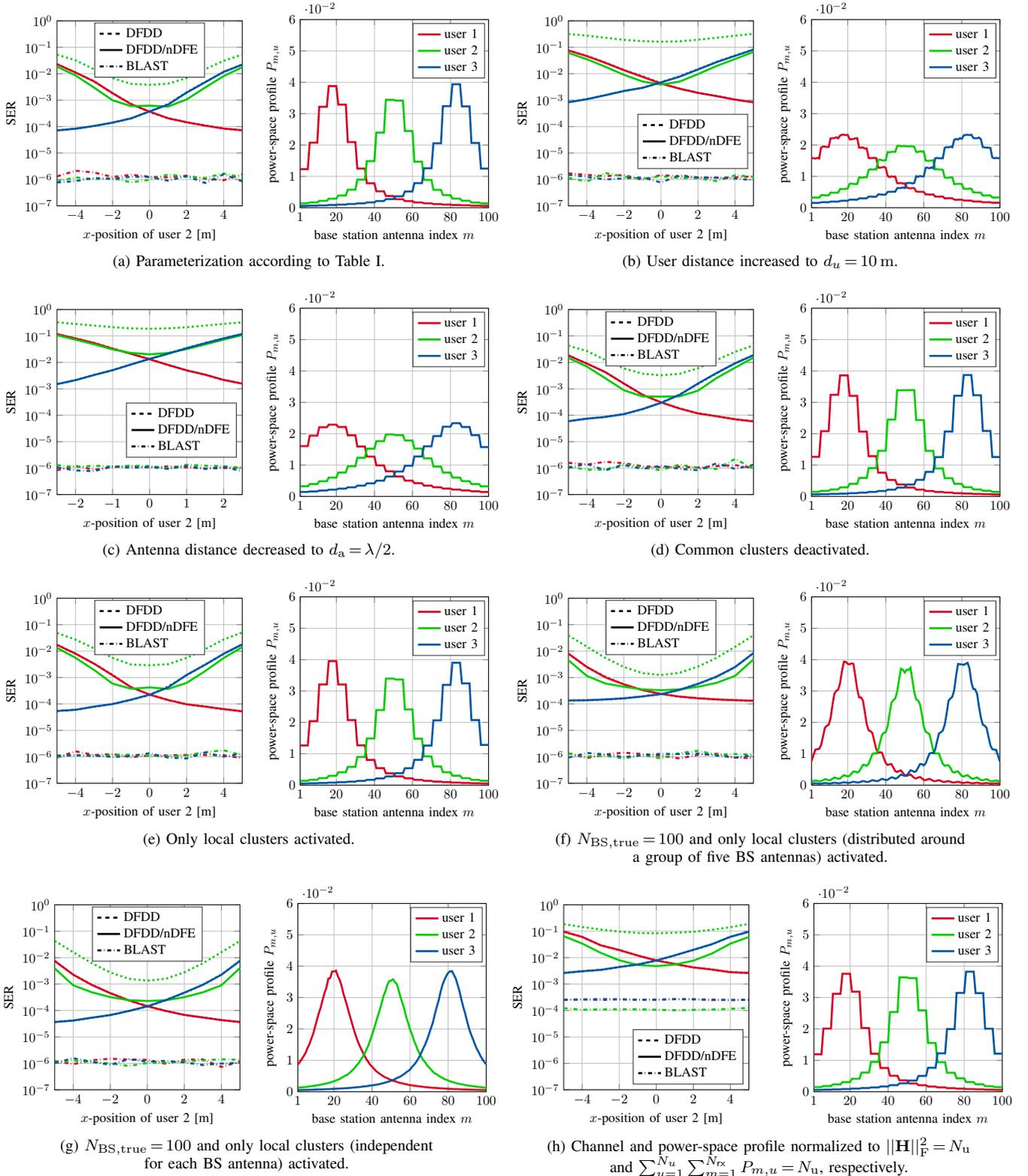
Fig. 4. Symbol error rate vs.  $x$ -position of user 2 (colors correspond to users: user 1 (—), user 2 (—), user 3 (—)) and power-space profile at zero  $x$ -position of user 2. Parameterization according to Table I.
