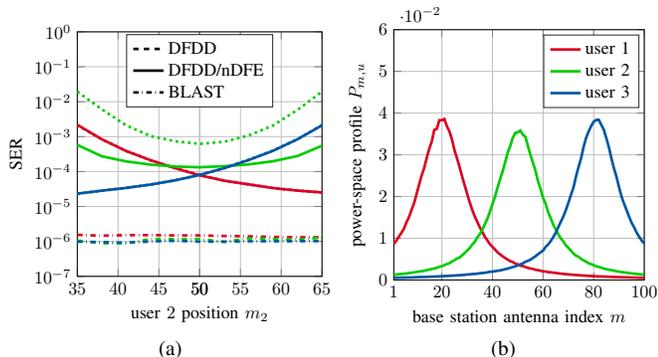
Fig. 6. (a) Symbol error rate vs. user 2 position  $m_2$  using idealized channel model in [6] (colors correspond to users: user 1 (—), user 2 (—), user 3 (—)) and (b) power-space profile at  $m_2 = 50$ , which is taken from the COST 2100 channel model evaluation of Fig. 4g.
