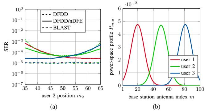
Fig. 5. (a) Symbol error rate vs. user 2 position  $m_2$  using idealized channel model in [6] (colors correspond to users: user 1 (—), user 2 (—), user 3 (—)) and (b) power-space profile at  $m_2 = 50$ . Parameterization adapted to Table I of COST 2100 channel model evaluation,  $\gamma = 3.6$  and  $\zeta^2 = 77$ .
