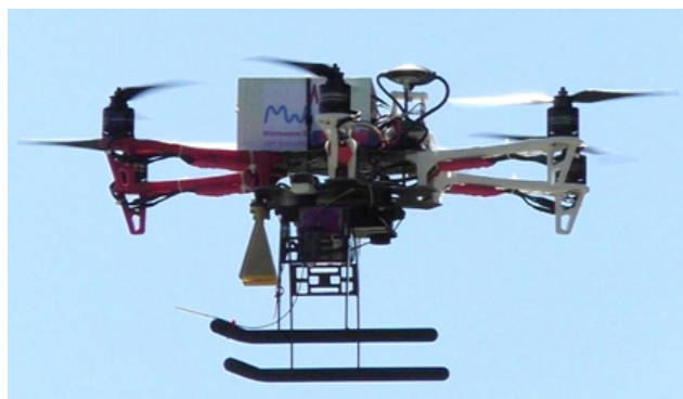
Figure 1. Picture of the hexacopter with mounted radar altimeter.
