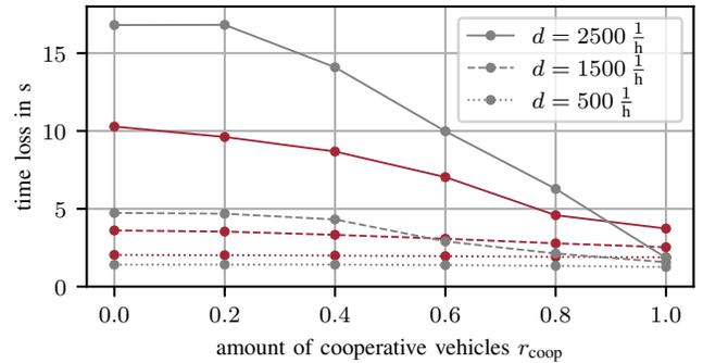
Fig. 7. Average time loss  $L(V)$  at the intersections in Aachen (red) and Ulm-Lehr (gray). 1000 approaching vehicles were spawned randomly with varying traffic density  $d$  and increasing cooperative vehicle ratio  $r_{\text{coop}}$ .
