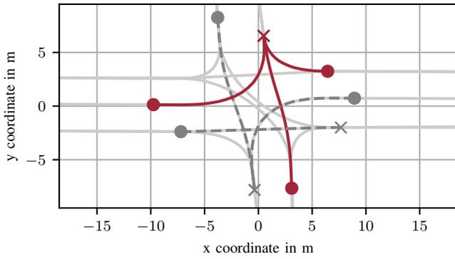
Fig. 2. Intersection at Bendplatz (Aachen, Germany) with a horizontal main road that has separate left turn lanes. This figure shows all lanes (light gray) and two exemplary conflict zones at crossing (dark gray, dashed) and merging (red) lanes, including their start (circle) and end (cross) points.
