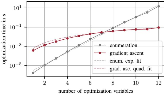
Fig. 5. Average computation time for finding the optimal maneuver using the enumeration and gradient ascent algorithms depending on the number of cooperative vehicle pairs, and respective exponential and quadratic fits.
