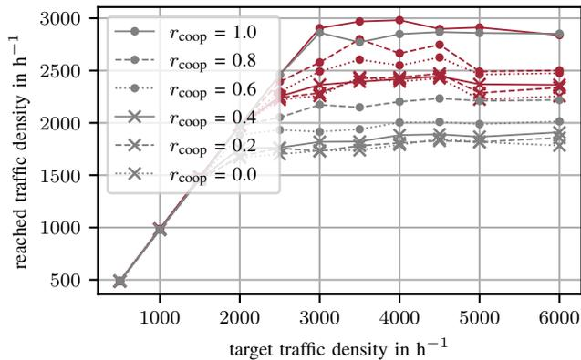
Fig. 9. Reachable traffic throughput at the intersections in Aachen (red) and Ulm-Lehr (gray), averaged over 1000 random vehicles, with varying cooperative vehicle ratio  $r_{\text{coop}}$  and an increasing target traffic density.
