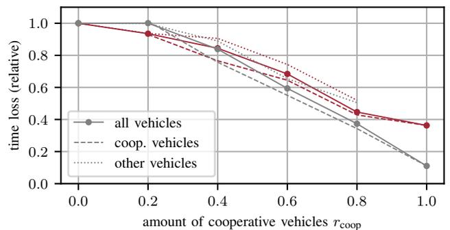
Fig. 8. Relative effect of cooperative maneuvers on the average time loss  $L(V)$  at the intersections in Aachen (red) and Ulm-Lehr (gray), with 1000 random vehicles at a traffic density of  $d = 2500 \frac{1}{h}$  and increasing cooperative vehicle ratio  $r_{\text{coop}}$ .
