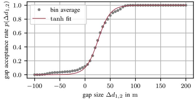
Fig. 3. Gap acceptance between two vehicles approaching an intersection as observed in the SUMO simulator.  $p(\Delta d_{1,2}) = p(d_2 - d_1)$  is the probability of vehicle  $V_1$  on a side road taking precedence over  $V_2$  on the main road. The figure shows acceptance rates averaged over bins and a tanh model.
