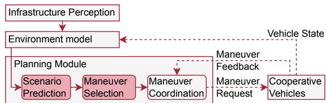
Fig. 1. Cooperative planning context overview. This work focuses on the scenario prediction and maneuver selection modules described in Section II and evaluated in Section III. V2X communication is marked dashed.
