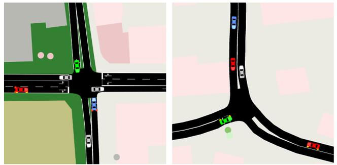
Fig. 6. Unsignalized intersections used for evaluation in SUMO [20]. Left scene (Bendplatz, Aachen): horizontal main road with separate left turn lanes. Right scene (Loherstraße, Ulm-Lehr): bending main road and side road from the left. Gray vehicles are not cooperative, blue ones are cooperative but not in a maneuver. Red vehicles yield to the prioritized green one to lower the average crossing duration.
