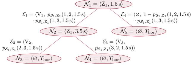
Fig. 4. Exemplary decision tree at  $t = 0$  where vehicles  $V_1, V_2, V_3$  approach the conflict zone  $Z_1$ . Edge  $\mathcal{E}_4$  is not explored further, so it directly ends with a leaf node without any further intermediate nodes. Decision trees in the evaluation scenarios have a much higher number of nodes and edges.
