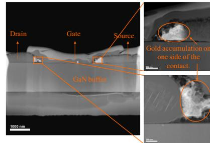
Fig. 3 High-Angle Annular Dark Field (HAADF) Scanning Tunneling Electron Microscopy (STEM) image of cross section of the device after 30 min annealing at 800 °C. Gold accumulation on one side of the ohmic contact could be identified.
