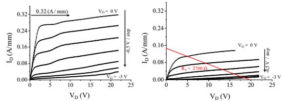
Fig. 6 Output characteristics of the InAlN/GaN HEMT. Left: device at R.T.; Right: device at 800 °C. Also shown the load line selected for 800 °C operation experiment.
