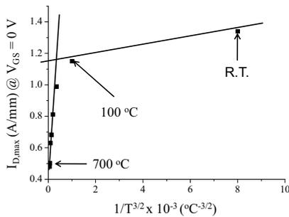
Fig. 8 Maximum output current density in dependence on the operation temperature.
