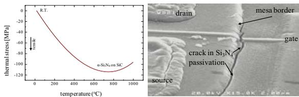
Fig. 5 Left: Thermal stress of Si<sub>3</sub>N<sub>4</sub> on SiC substrate. Right: Crack in Si<sub>3</sub>N<sub>4</sub> passivation due to high tensile stress at elevated temperature.
