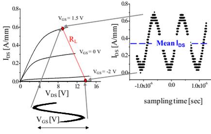
Fig. 1 Test arrangement of temperature stepping experiment. Input signal 1 MHz; bias point and amplitude adjusted as shown. Output termination by  $R_L$ . Output and input wave form recorded every 60 sec.
