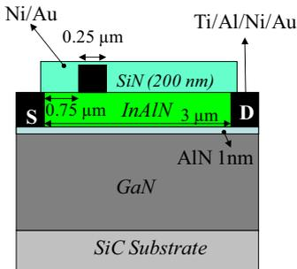
Fig. 2 General cross section of devices used.
