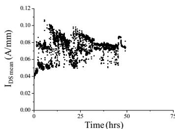
Fig. 9 Up to failure high temperature cycling of InAlN/GaN HEMT with Cu based metallization. 900 °C step shown.
