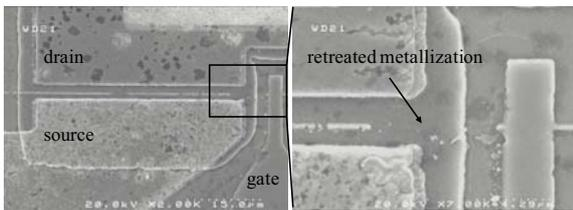
Fig. 4 Topography of InAlN/GaN HEMT after failing during 900 °C large signal RF operation.
