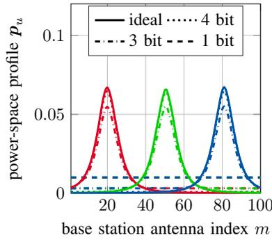
(a) Normalized effective power-space profile  $\hat{p}_u$  at different resolution of the ADCs.
