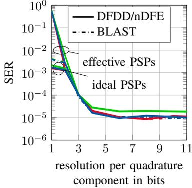
(b) Symbol error rate vs. resolution of the ADCs for  $E_{s,tx}/N_0 \approx 14$  dB.
