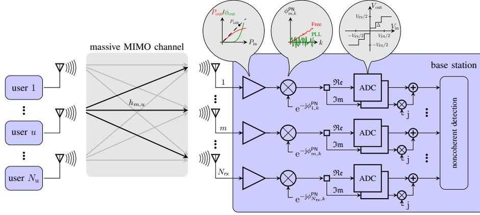
Fig. 1. Generic system model for the massive MIMO uplink transmission including the main hardware components at the base station.
