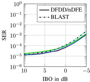
Fig. 3. Symbol error rate vs. IBO of a non-linear amplifier based on a fifth-order polynomial as in [26] for  $E_{s,\text{tx}}/N_0 \cong 14$  dB. Colors correspond to users: user 1 (—), user 2 (—), user 3 (—).
