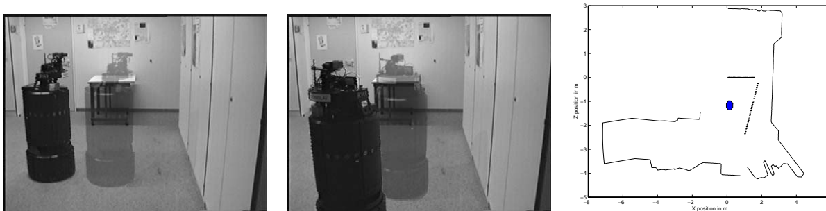
Figure 7: Experiment showing successful collision avoidance. The obstacle (wall) is detected from the TTC values in the central sector. Left : Two superimposed snapshots before the turn. Middle : Two superimposed snapshots after the turn. Right : Robot trajectory from odometry (dotted) and environment (from laser scan)
