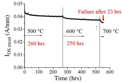
Fig. 10. Test cycles of InAlN/GaN HEMT up to failure. Failure occurred after 23 h at  $700 \text{ }^\circ\text{C}$ .
