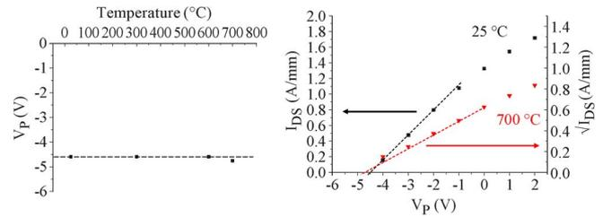
Fig. 11. (Left) Change of extracted pinchoff voltage (see right) at operating temperature of  $L_g = 0.25 \mu\text{m}$  FET. (Right) Extraction of pinchoff voltage at the onset of saturation: At  $25 \text{ }^\circ\text{C}$  from linear transfer characteristic (high-mobility short-channel case) and at  $700 \text{ }^\circ\text{C}$  extraction from the square root plot of the transfer characteristics (low-mobility long-channel case).
