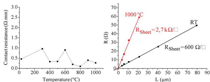
Fig. 4. (Left) Change of contact resistance with operating temperature. (Right) Extrapolation of planar contact resistance and sheet resistance from TLM measurements at measurement temperatures of RT and 1000 °C.
