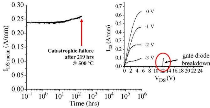
Fig. 8. Failure cycle of AlGaIn/GaN HEMT device as described in the text. Operation conditions:  $R_L = 500 \Omega$ ,  $V_{DS} = 20 \text{ V}$ ,  $V_{GS} = -3.6\text{--}0 \text{ V}$ ,  $f_{in} = 1 \text{ MHz}$ , and temperature stepping from  $300 \text{ }^\circ\text{C}$  to  $500 \text{ }^\circ\text{C}$ .
