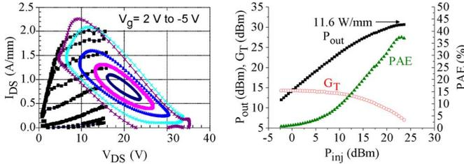
Fig. 6. Large-signal 4-GHz power performance of InAlN/GaN MISHEMT structure, including hard input overdrive conditions. Device data:  $t_{\text{InAlN}} = 10$  nm,  $T_{\text{oxide}} = 1.5$  nm,  $L_G = 0.25$   $\mu\text{m}$ , and  $W_G = 2 \times 50$   $\mu\text{m}$ . In part after [48].
