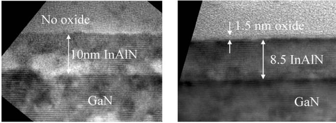
Fig. 5. TEM cross section of lattice-matched InAlN/GaN heterostructure with 10-nm barrier thickness. (Left) Heterostructure before oxidation. (Right) Heterostructure after oxidation at 800 °C in O<sub>2</sub> for 4 min [46].
