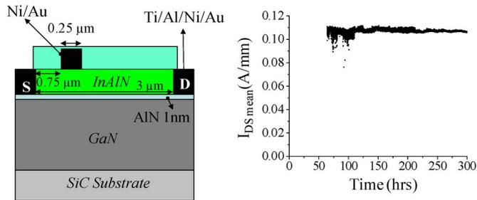
Fig. 9. (Left) Device cross section of the InAlN/GaN HEMTs. First- and second-generation devices differ only in the ohmic and gate contact metallization schemes. (Right)  $500 \text{ }^\circ\text{C}$  test step of a typical InAlN/GaN device with lattice-matched barrier layer.
