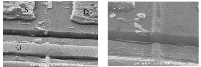
Fig. 16. Topography of InAlN/GaN HEMT after failing at 900 °C large-signal RF operation. (Left) After removal of Si<sub>3</sub>N<sub>4</sub> passivation. (Right) Passivated.
