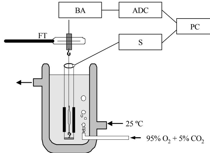
**Figure 5: Scheme of the setup used for the force recordings in muscles.**
