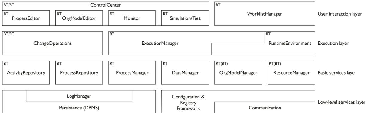
Figure 13: Basic Architecture of ADEPT2 (BT: Buildtime; RT: Runtime)
